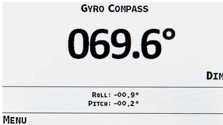
Figure 3-2 Start Screen on Operating Unit
