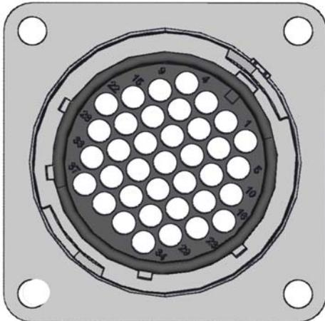
Figure 1-6 Sockets of Data Interfaces N1 and N2
